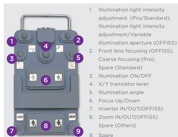
Footswitch layout with well-accepted control configuration.
